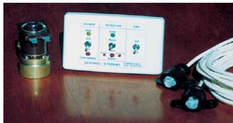
Gas detection equipment
