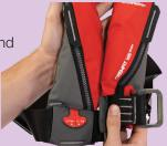
Following the manufacturer's instructions reveal the inflation system and oral inflation tube. Inflate the bladder using the oral tube and leave overnight in a room with a constant temperature. If the bladder loses pressure, immediately take the jacket to an accredited service agent for further
