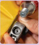
be replaced immediately. On auto inflation jackets also ensure the auto components are armed and in date. Refit the cylinder to inflation system, tightening it by hand until firm. Do not over tighten.
